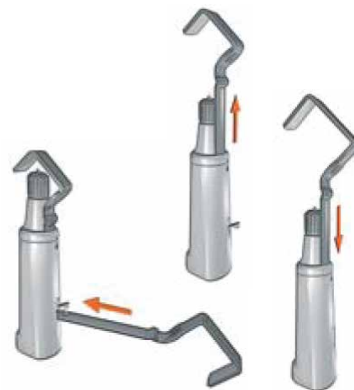
Cable size range per clamp: 0.18" - 1.0" / 4.5 mm - 25 mm 0.8" - 1.5" / 20 mm - 40 mm
